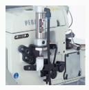
Pressing the treadle with your heel raises the presser foot. This device is easy to use, thus decreasing operator fatigue and increasing productivity.
