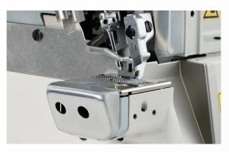
Thanks to the independently driven top feed mechanism, feeding efficiency has been increased dramatically. This feature responds to a wide variety of fabrics, including light to heavy weight fabrics.
